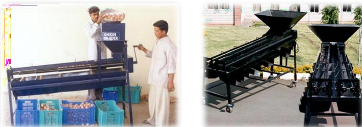
Fig.8. Onion grader developed by ICAR-DOGR
