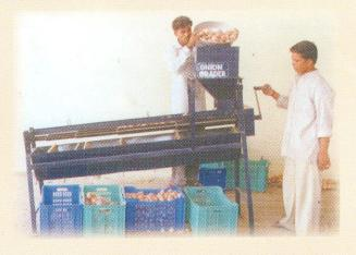
NRC Onion & Garlic developed roller type onion grader. This has a capacity of 0.5 t /h/labour as compared to 0.1 t/h/labour in manual grading. It grades onion in five different grades (< 35, 35-50, 50-60, 60-80 and > 80 mm) according to the size of the bulbs. It is manually operated but can be motorized. The grader has total weight of 50 Kg and can easily be taken to fields. The grader has 10 times higher precision than manual grading.
